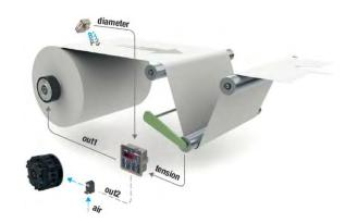
Regulation in torque with load cells or dancer roller
